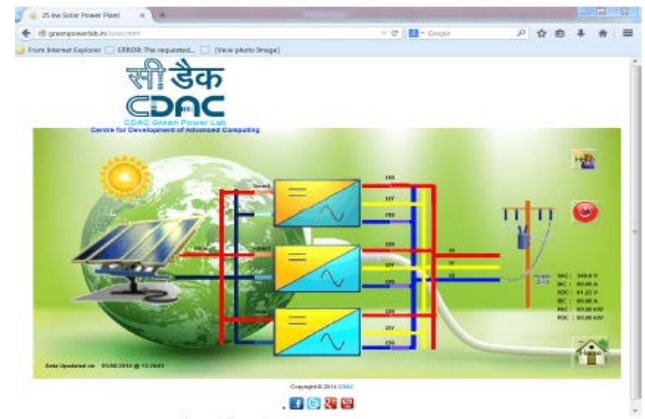
Fig. 2.8 Screen shot of on-line HMI
